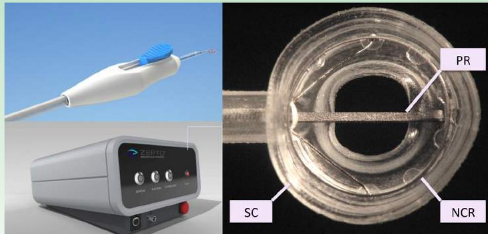
The Zepto capsulotomy system consists of a disposable handpiece attached to a control console that provides power and suction for the capsulotomy (left). The handpiece terminates in a soft, clear silicone capsulotomy tip that houses a circular collapsible super elastic nitinol ring to perform the capsulotomy (right).
